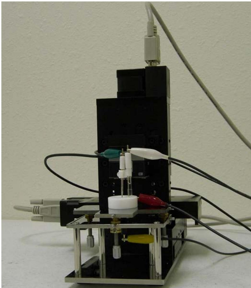
Figure 2.3. Nanopositioner and Cell/sample holder
