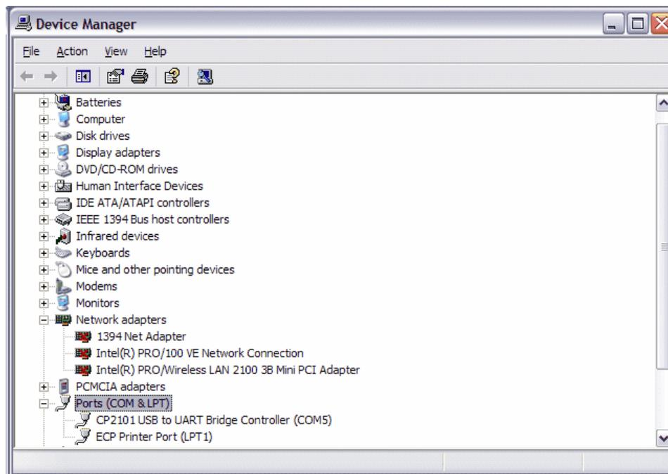
7. Determine the COM number for the newly installed "CP2101 USB to UART Bridge Controller" or similarly named device.
