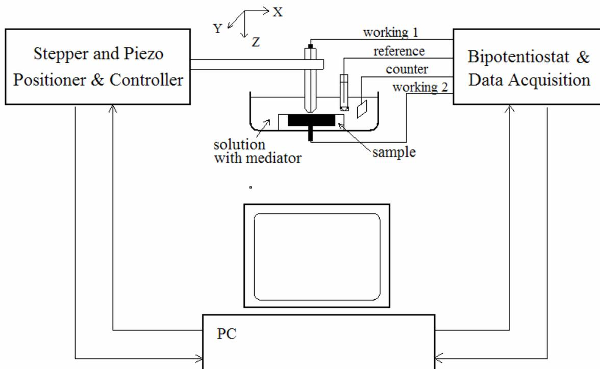
The model 900D/920D is designed for scanning electrochemical microscopy, but is also capable of many conventional electrochemical techniques for convenience.
