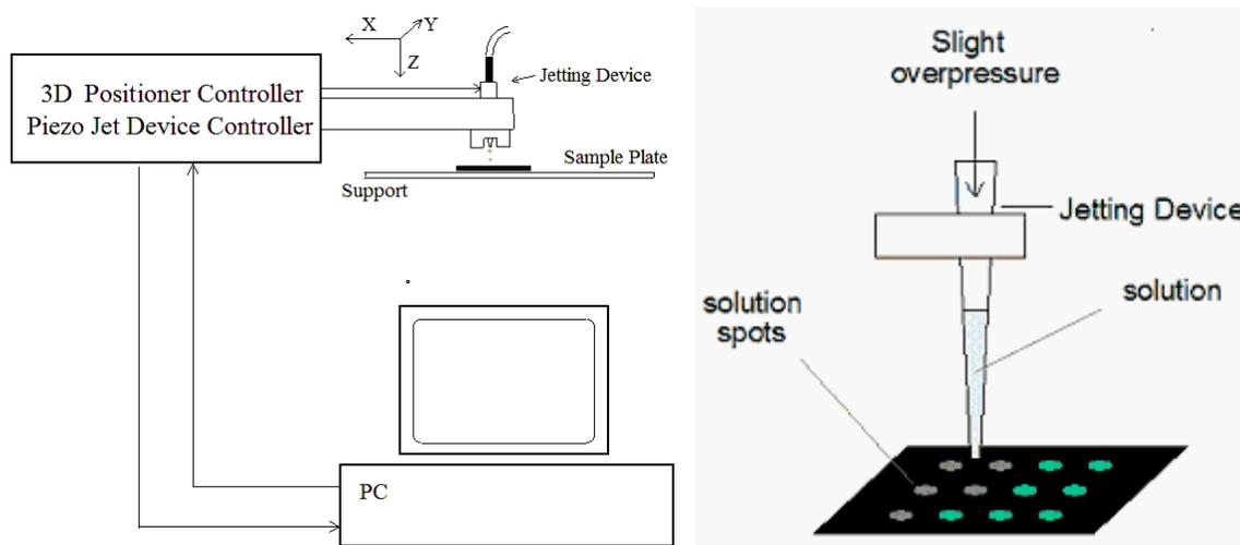
**Figure. Diagram of the solution dispenser**
