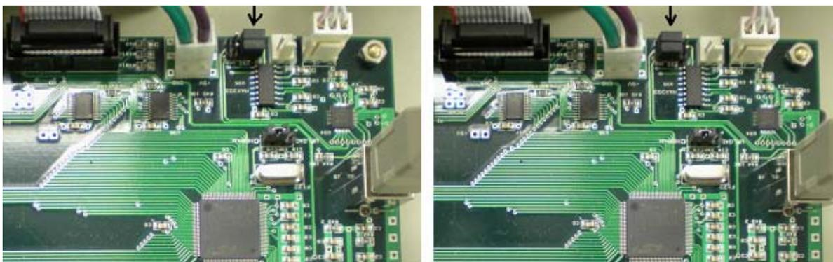
**Figure 2.2** Serial port or USB port switch selection using two jumpers (indicated by arrows). Left: RS-232 serial port jumper setting. Right: USB jumper setting.
