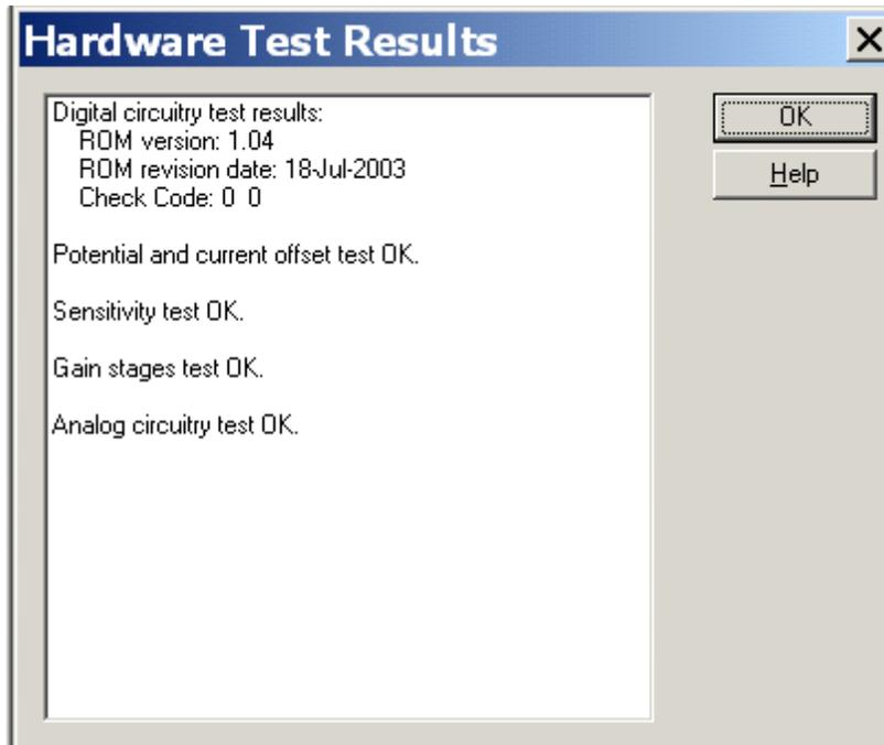
Review the Self Test results carefully. In the case of an analog test error, please repeat the test several times to see if the error is consistent. Record the error message and contact the factory for servicing.
