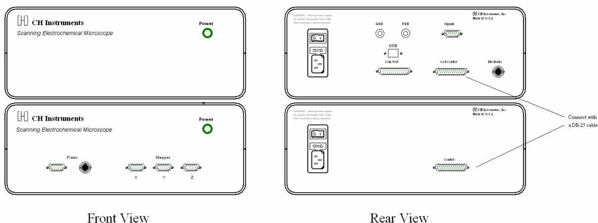
**Figure 2.1. Front and rear view of the instrument chassis for the stepper motor/piezo controller (bottom) and bipotentiostat (top).**
